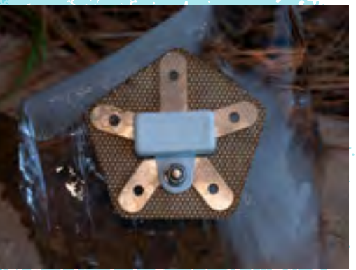
BURR ON FUR Polar bears at the San Diego Zoo are helping their cousins on the tundra and sea ice by testing out a new technology to track white bears across their vast, snowy habitat. Nicknamed "Burr on Fur," in this collaboration with Polar Bears International, 3M, and eight other zoos, scientists developed a small tracking device that temporarily attaches to bear fur. If successful, these small devices will significantly improve the ability to monitor polar bears in native habitats and determine how climate change is affecting their movements—vital information that will inform further work to save them.
